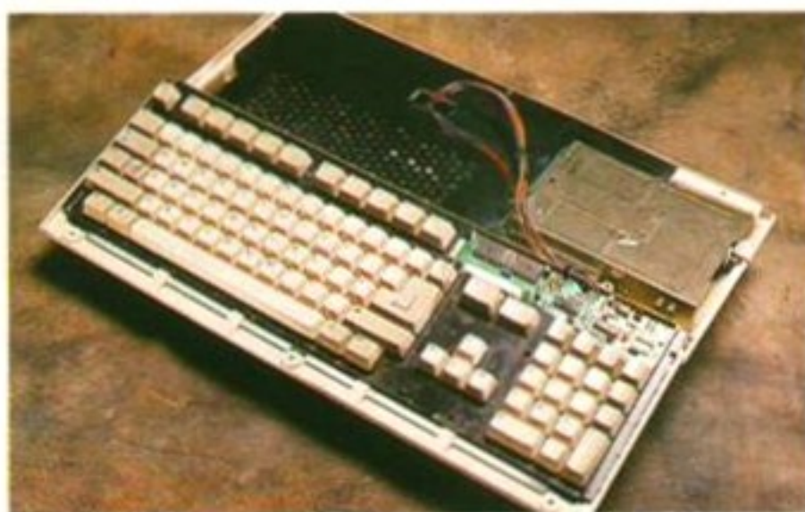
Yes, an Amiga with it's case off. There's still a metal shield left to get through at this stage.
